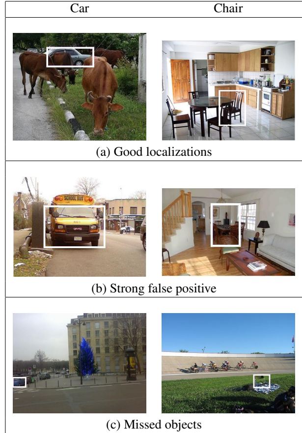
Figure 4. Localization examples for the classes car and chair with our detector ( \chi^2 , HOG + BOF) on PASCAL VOC 2007. (a) Examples of objects correctly detected. (b) Examples of false positives with high score. (c) Examples of objects that were missed.
